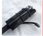
Above: With the metal cover removed the viewer can see the four coloured wires going to the contact board, along with the black earth.
