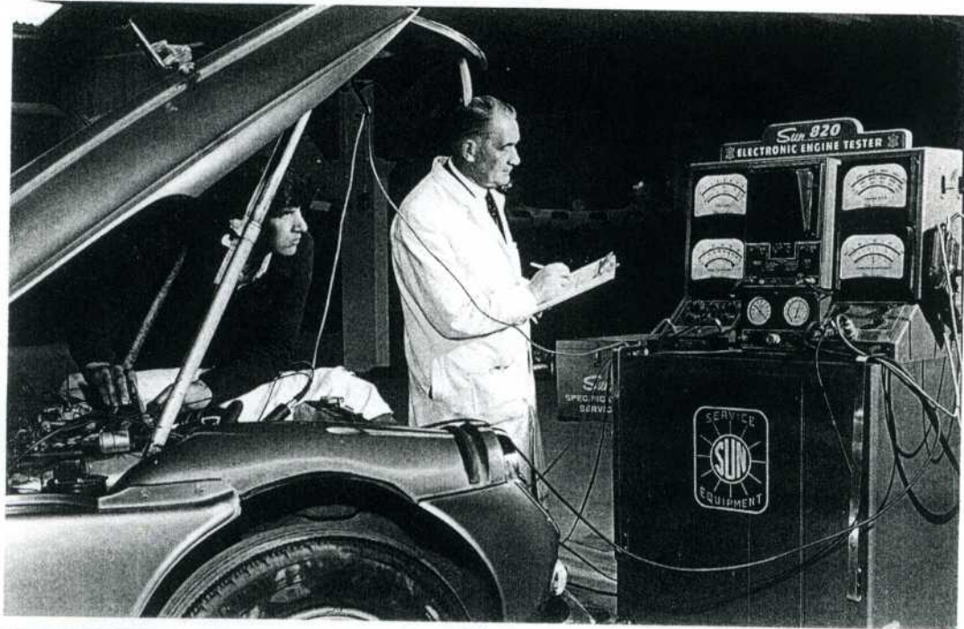
Yet another example of Jensen's desire to be at the forefront of technology. A C-V8 engine being set up on a Sun electronic engine tester.
