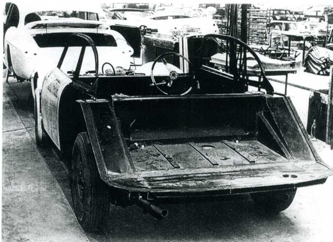
The C-V8 production line showing the main body assembly. Austin Healey bodies can be seen in the background.
