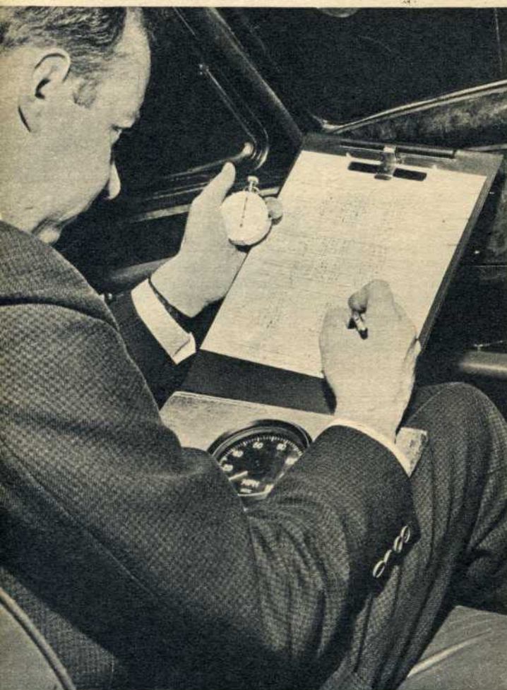
Acceleration: an observer notes times from the recording stopwatch after a run. Between his legs is the head of the electric speedometer
