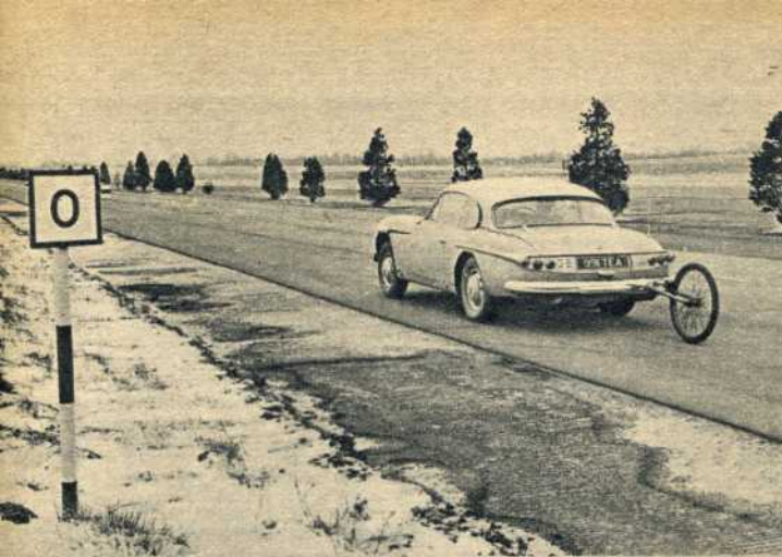
Acceleration: at the start of the quarter-mile on the M.I.R.A. No. 2 straight, the Jensen takes off trailing the electric fifth wheel for speed measurements. Several runs are made each way
