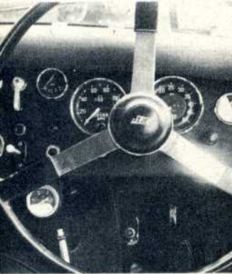
Dashboard is quite different though both models have the same instrumentation. The earlier 541 (bottom) has the better view from the driver's point of view with all instruments visible through the steering wheel and not masked as C-V8 ▼
