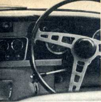
Dashboard is quite different though both models have the same instrumentation. The earlier 541 (bottom) has the better view from the driver's point of view with all instruments visible through the steering wheel and not masked as C-V8 ▼
