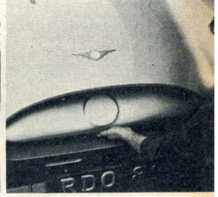
▲ Front styling is completely different. The 541 (bottom) has a unique swivelling panel to control the amount of cooling air going into the grille and twin headlamps. The C-V8 has a shallow wide grille with rather ugly four-headlamp system ▼
