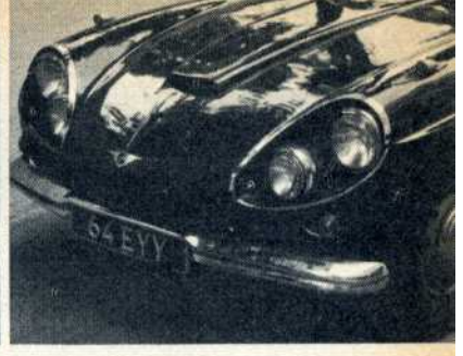
▲ Front styling is completely different. The 541 (bottom) has a unique swivelling panel to control the amount of cooling air going into the grille and twin headlamps. The C-V8 has a shallow wide grille with rather ugly four-headlamp system ▼
