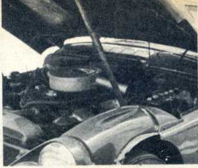
▲ Engine compartments are similar with same sort of bonnet, but the works are completely different. The C-V8 (top) has the Chrysler V8 engine for more performance, whilst the 541 has the smaller Austin six-cylinder unit for better mpg ▼
