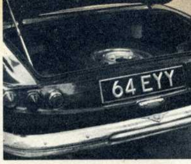
▲ Boot space is limited on both models considering the car is designed for long distance touring, but the 541 (bottom) has easier access with the lid coming right down to the boot floor level. The C-V8 has more up-to-date rear lights layout ▼
